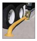
As the vehicle approaches the loading dock, it is guided into position between the wheel guides. The rearmost tyre makes contact with the restraint's trigger device.
