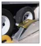
The trigger device then moves towards the loading dock, using the energy of the trailer. The locking arm determines the size of the tyre automatically, rising to its full height against the wheel.
